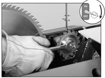
Figure 34. Installing the scoring blade.
